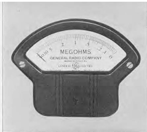
FIGURE 4. View of the meter scale. Except at the low end of the lowest range and at the high end of the highest range, only the center decade of the scale needs to be used.
